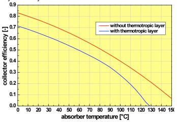
Fig. 2. Effect of thermotropic layer on collector efficiency and maximum absorber temperature of an all-polymeric solar collector with twin-wall sheet glazing and black absorber ( $\alpha$ =0.95,  $\varepsilon$ =0.90) at a solar irradiation of 1000 W/m<sup>2</sup> and an ambient temperature of 20 °C.
