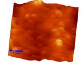
Fig. 5: Topography of unaged PPS (left), after 500 h UV irradiation (middle) and 500 h at 85 °C, 85% r.h. (right).
