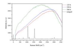
Fig. 4: Raman-spectra of PPS, after different times of exposure to UV irradiation.
