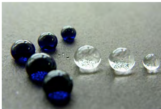
Fig. 3. Water drops on surface of the TISS paint coating.
