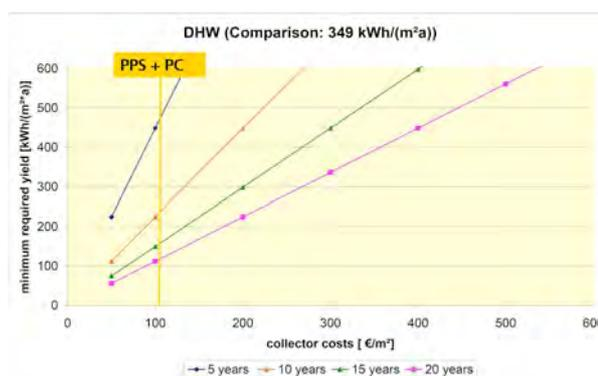
assumed polymeric and an average conventional collector. On the other hand, the required minimum yield was estimated in relation to the lifetime and costs of the collector. It could be shown that, under certain assumptions, polymeric collectors can economically compete with conventional ones.
