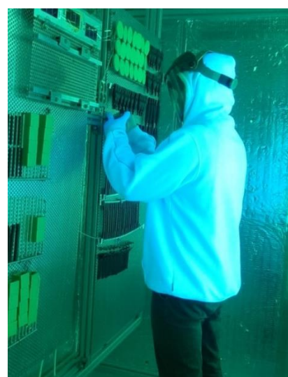
Figure 1: left: Comparison of the spectral intensity distribution of different light sources for UV aging. It shows not only a broad variation in total intensity, but also in regions of the UV range. Right: Researcher in protective gear sampling different polymer specimen in a UV chamber.
