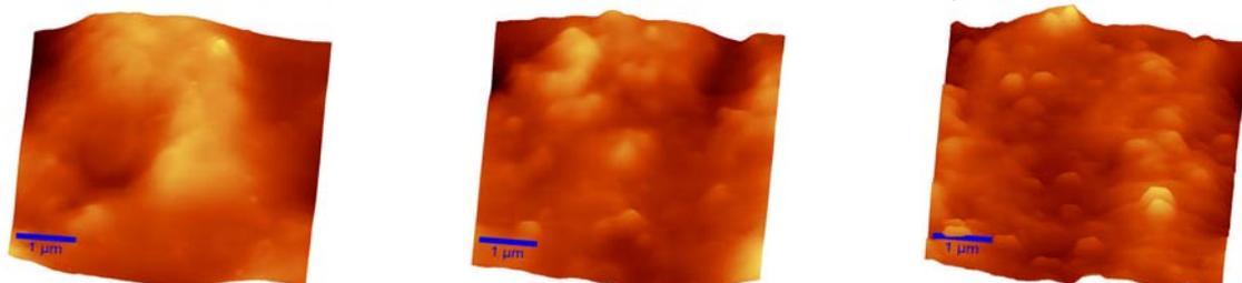
Fig. 5: Topography of unaged PPS (left), after 500 h UV irradiation (middle) and 500 h at 85 °C, 85% r.h. (right).
