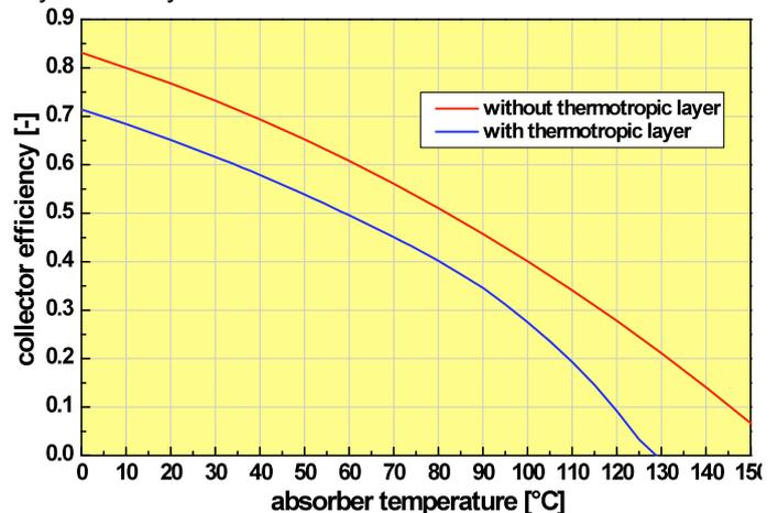
Fig. 2. Effect of thermotropic layer on collector efficiency and maximum absorber temperature of an all-polymeric solar collector with twin-wall sheet glazing and black absorber ( $\alpha=0.95$ ,  $\epsilon=0.90$ ) at a solar irradiation of 1000 W/m<sup>2</sup> and an ambient temperature of 20 °C.
