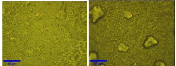
Fig 3: Micrographs of unaged PPS (left) and after 500 h UV irradiation (right).
