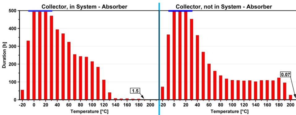
Fig. 2. Distribution of the annual temperature loads on the absorber in the system (left) and not in the system (right)
