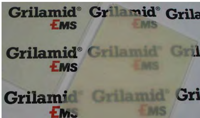
Fig. 4. Thermotropic polyamide in clear and scattering state (left) and AFM phase image representing layer morphology (right).
