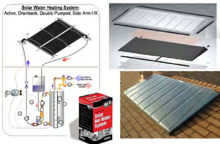
Fig. 1. The FAFCO drainback system is shown schematically on the left. It uses unglazed collectors in a drainback system, and the system's storage is shipped in a small UPS container. The DEG/Harperis Energy system is shown on the right. It has an immersed heat exchanger in a glazed or unglazed polymer tank.
