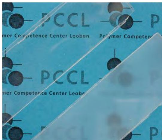
Thermotropic layer developed at the PCCL in clear (left) and scattering state (right).
